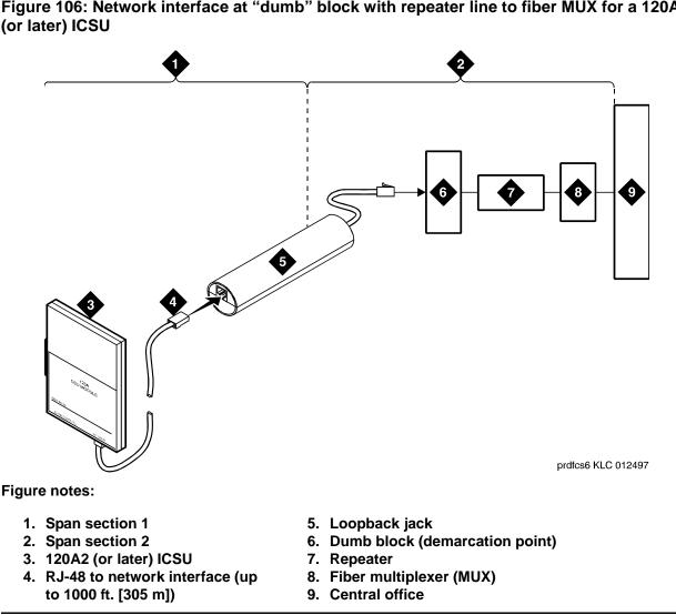
Figure 106: Network interface at "dumb" block with repeater line to fiber MUX for a 120A2 (or later) ICSU
